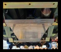
Made up in alluminium 10mm thickness, very heavy duty protection
