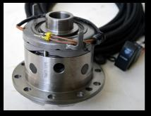
Air/e-lockers allow to lock differential when car is on hard sand/mud; working is excellent both air or electrical type on front and rear axle
