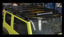
All plates are 5mm thickness, squared brackets in 35x35x3, 6 fitting points to the roof, easy fit on top; made up in steel, black powder coated
