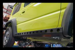
Thickness 6mm, folded and renforced inside, very heavy duty and great looks for Jimny; black powder coated
