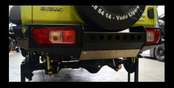
Thickness steel plates 5mm, low alluminium manifold skid plate included; black powder
